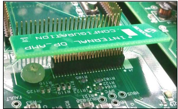
FIGURE 1: INTERNAL OP AMP CONFIGURATION BOARD
