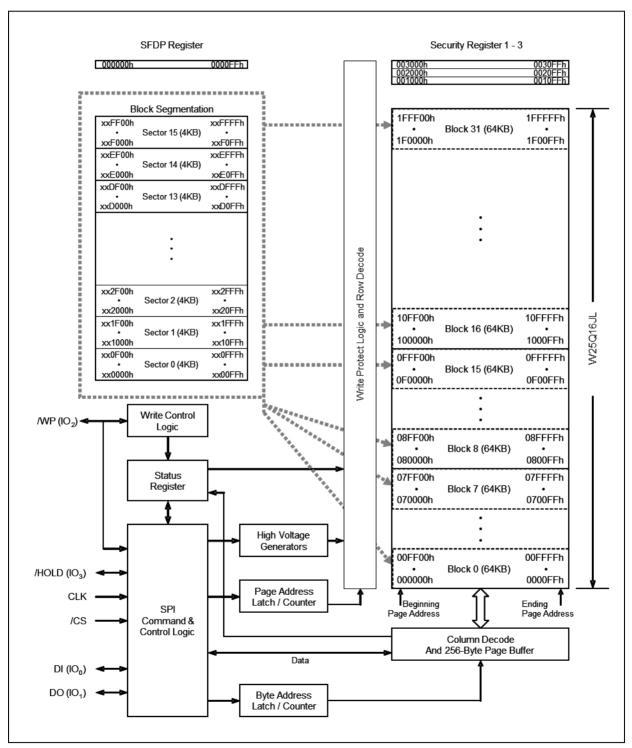
Figure 2. W25Q16JL Serial Flash Memory Block Diagram
