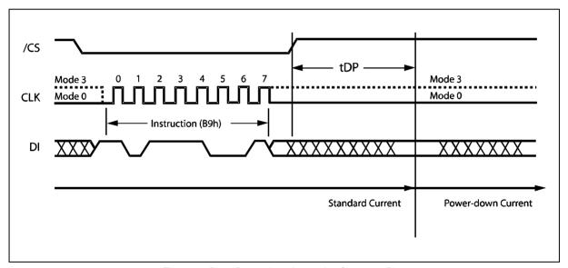
Figure 27. Deep Power-down Instruction Sequence Diagram
