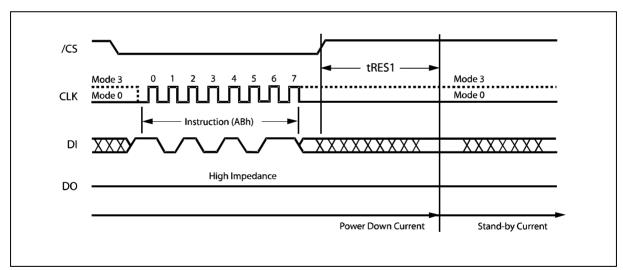
Figure 28a. Release Power-down Instruction Sequence
