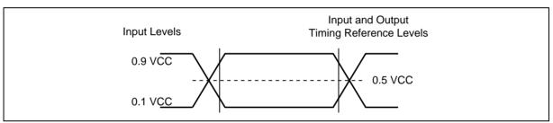
Figure 60. AC Measurement I/O Waveform
