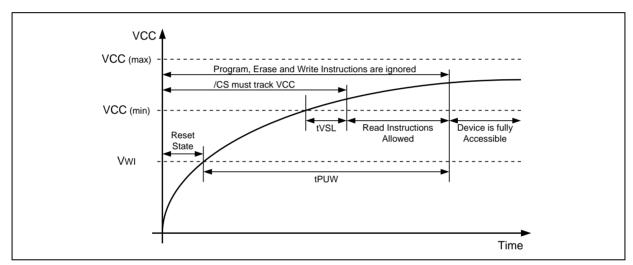
Figure 59a. Power-up Timing and Voltage Levels
