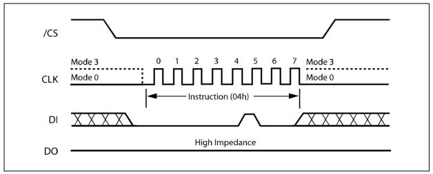
Figure 6. Write Disable Instruction Sequence Diagram
