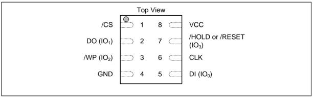
Figure 1b. W25Q16JL Pad Assignments, 8-pad WSON 6x5-mm, USON 2X3-mm (Package Code ZP, UX)
