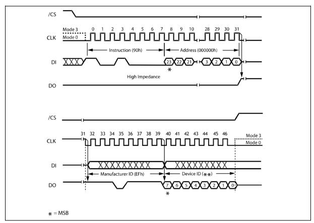
Figure 29. Read Manufacturer / Device ID Diagram
