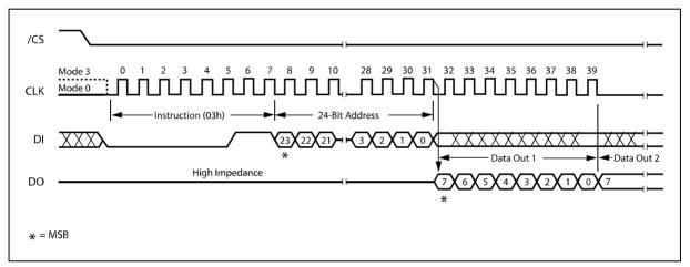
Figure 9. Read Data Instruction Sequence Diagram
