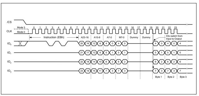
Figure 15a. Fast Read Quad I/O Instruction (Initial instruction or previous M5-4≠10, SPI Mode)
