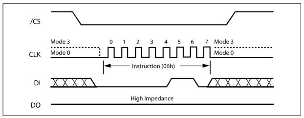
Figure 4. Write Enable Instruction Sequence Diagram
