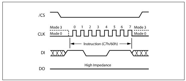
Figure 24. Chip Erase Instruction Sequence Diagram
