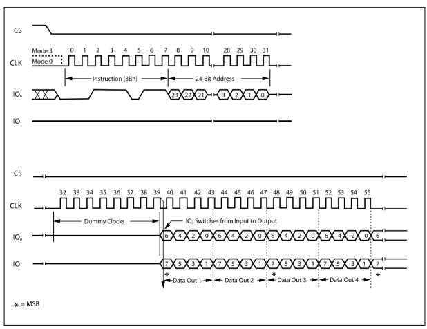
Figure 11. Fast Read Dual Output Instruction Sequence Diagram
