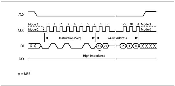
Figure 22. 32KB Block Erase Instruction Sequence Diagram
