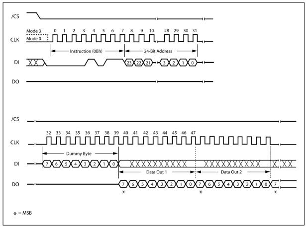
Figure 10. Fast Read Instruction Sequence Diagram
