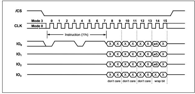
Figure 17. Set Burst with Wrap Instruction Sequence
