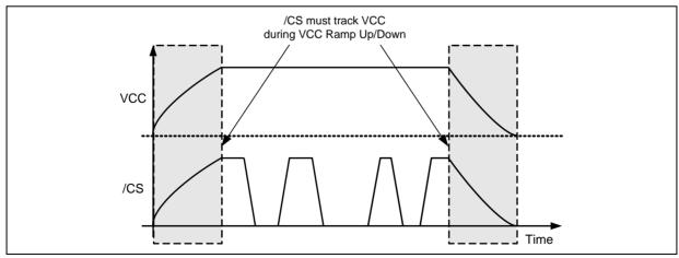
Figure 59b. Power-up, Power-Down Requirement
