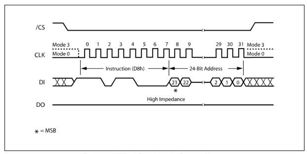
Figure 23. 64KB Block Erase Instruction Sequence Diagram
