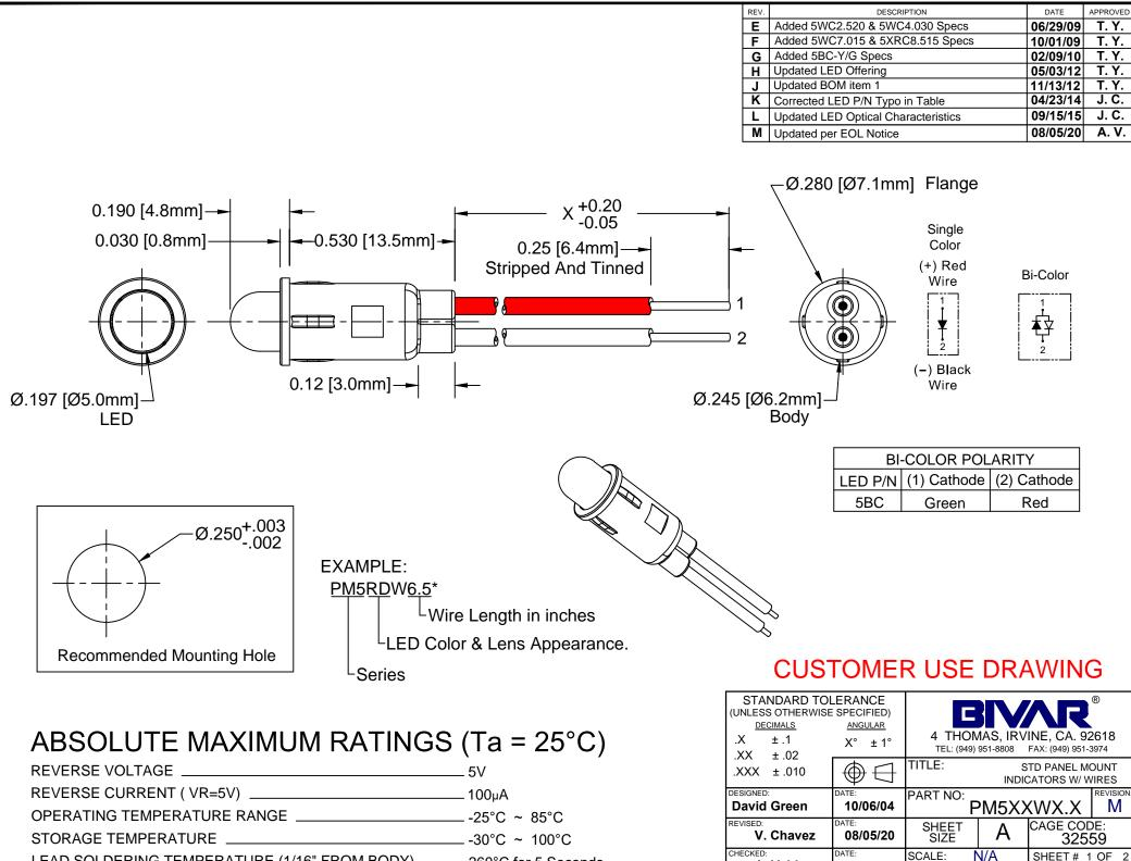
LEAD SOLDERING TEMPERATURE (1/16" FROM BODY) 260°C for 5 Seconds CHECKED: ATE: SCALE: N/A A. Valdez 08/05/20 CAD GENERATED DOCUMENT, DO NOT MEASURE DRAWING
