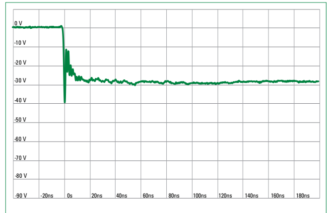
ISO10605 Contact Discharge Plot at -8 kV
