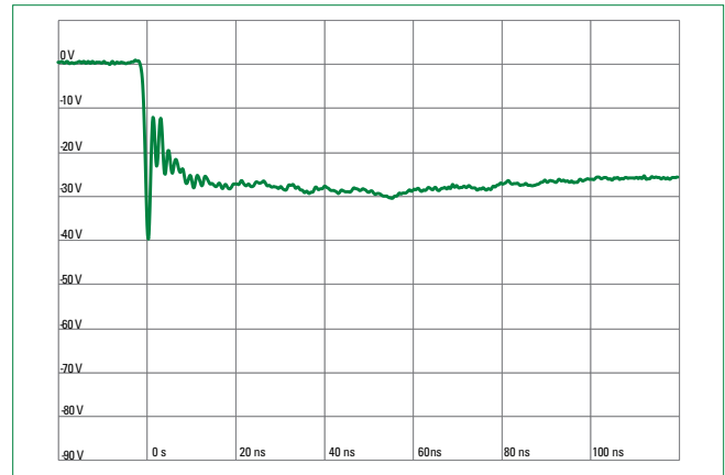
IEC 61000-4-2 -8 kV Contact ESD Clamping Voltage
