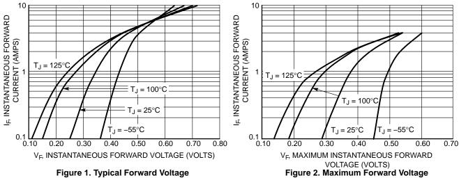
Figure 1. Typical Forward Voltage
