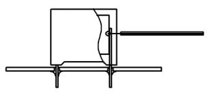
Temperature monitored inside the capacitor.
