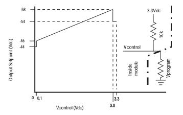
An open circuit on this pin sets the voltage level back to the original setting.
