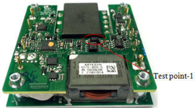
Figure 12: Temperature test point-1
