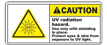
These products generate UVC radiation which can cause skin damage and conjunctivitis to humans and animals within a short time. The skin and eyes must be fully protected against exposure. You should be aware that UVC radiation does not eliminate harmful non-degradable substances such as heavy metals or pesticides. Assume IEC62471 Risk Group 3
