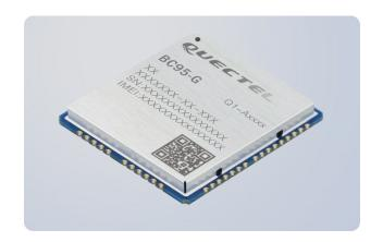
BC95-G is a high-performance NB-IoT module which supports multiple frequency bands of B1/B3/B8/B5/B20/B28 with extremely low power consumption. The ultra-compact 23.6mm × 19.9mm × 2.2mm profile makes it a perfect choice for size sensitive applications. Designed to be compatible with Quectel GSM/GPRS M95 module and NB-IoT BC95 module in the compact and unified form factor, it provides a flexible and scalable platform for migrating from GSM/GPRS to NB-IoT networks.
