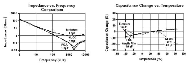
Type FCA capacitors have very low e.s.r. and stable capacitance vs. temperature.
