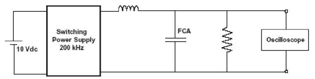
In the above circuit, one 1  $\mu$ F FCA capacitor results in the same ripple reduction performance as a 10  $\mu$ F tantalum capacitor at 200 kHz. With a 1  $\mu$ F tantalum capacitor in the circuit the measured ripple voltage was 70 mVpp, and with a 10  $\mu$ F tantalum or a 1  $\mu$ F FCA capacitor the ripple voltage was 8 mVpp.
