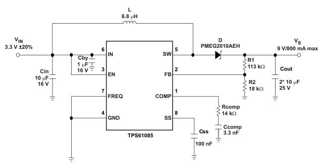
Figure 15. Typical Application, 3.3 V to 9 V ( $f_{sw}$  = 650 kHz)
