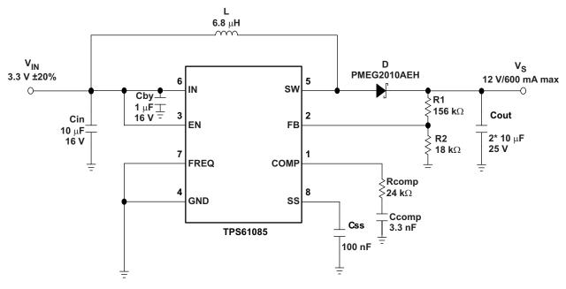
Figure 13. Typical Application, 3.3 V to 12 V ( $f_{sw} = 650 \text{ kHz}$ )
