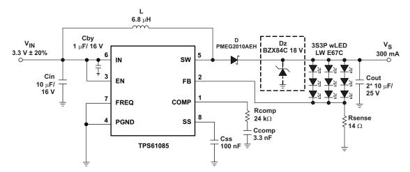
Figure 18. Simple Application (3.3V input -  $f_{sw}$  = 650 kHz) for wLED Supply (3S3P) (with optional clamping Zener diode)
