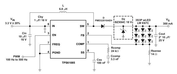
Figure 19. Simple Application (3.3V input -  $f_{sw}$  = 650 kHz) for wLED Supply (3S3P) with Adjustable Brightness Control using a PWM Signal on the Enable Pin (with optional clamping Zener diode)
