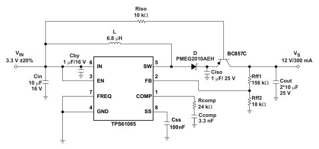
Figure 16. Typical Application with External Load Disconnect Switch
