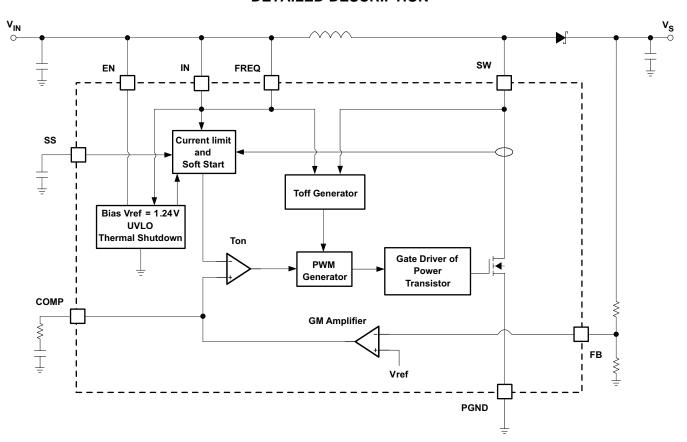
Figure 11. Block Diagram
