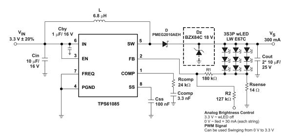
Figure 20. Simple Application (3.3V input -  $f_{sw}$  = 650 kHz) for wLED Supply (3S3P) with Adjustable Brightness Control using an Analog Signal on the Feedback Pin (with optional clamping Zener diode)
