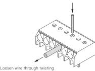
and pulling or using a  $\emptyset$  1mm release tool
