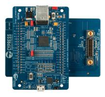
2. Connect the ON Semiconductor Image Sensor Board (MT9M114\_55CSP\_HB\_DEMO3\_REVO) to the CYUSB3ACC-004A Board
