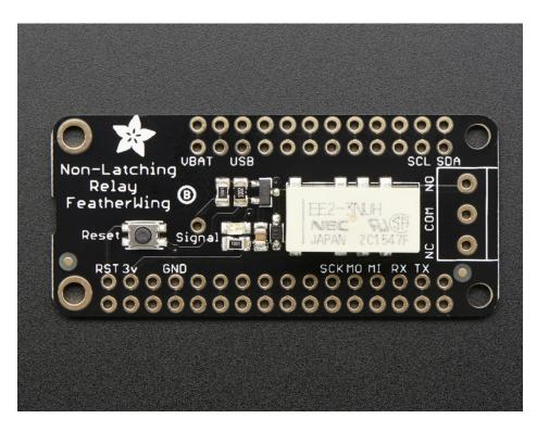
A Feather board without ambition is a Feather board without FeatherWings! These are the **Mini Relay FeatherWing**. They will give you power to control, and control over power. Put simply, you can now turn on and off lamps, fans, solenoids, and other small appliances that run on up to 250VAC or DC power using any Feather board.
