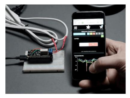
The are two 'flavors' of these FeatherWings, the first is the simple **Non-Latching** relay. This Wing has a single Set pin.
