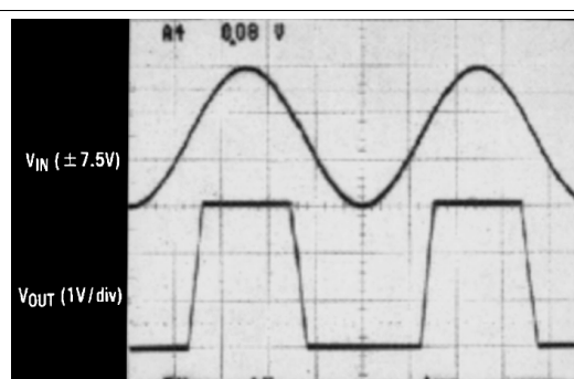
A \pm 7.5 -V input signal greatly exceeds the 3-V supply in Figure 63 causing no phase inversion due to R_I .
