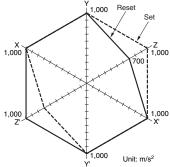
Sample: G6BK-1114P-US Number of Relays: 12 pcs Test Conditions: The value at which malfunction occurred was measured after Shock direction applying shock to the test piece 3 times each in 6 directions along 3 z 💿 axes. Standard value: (Coil) 300 m/s<sup>2</sup>
