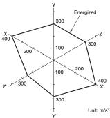
Sample: G6B-1114P-US Number of Relays: 12 pcs Test Conditions: Shock is applied in  $\pm X$ ,  $\pm Y$ , and ±Z directions three times each with without energizing the Relays Shock direction X → X to check the number of malfunctions. z 💿 Requirement: None malfuction 100 m/s² (Coil)
