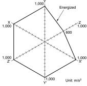
Sample: G6B-1174P-US G6B-1174P-FD-US Test Conditions: Shock is applied in ±X, ±Y, and ±Z directions three times each with without Shock direction energizing the Relays to check the number of malfunctions. Requirement: None  $Z' \otimes$ malfuction 100 m/s2 (Coil)
