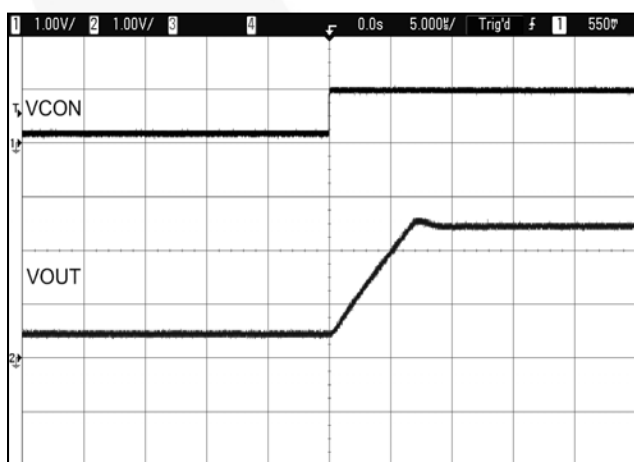
Figure 38. V_{OUT} Rising Transition 0.5 V to 3.0 V, V_{IN} = 3.7\text{ V} in High-Power Mode
