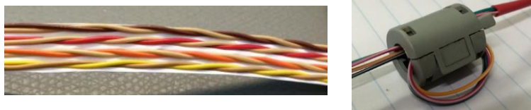
Figure 164: Example of Twisted Pair Cable with 4 Pairs and Ferrite
