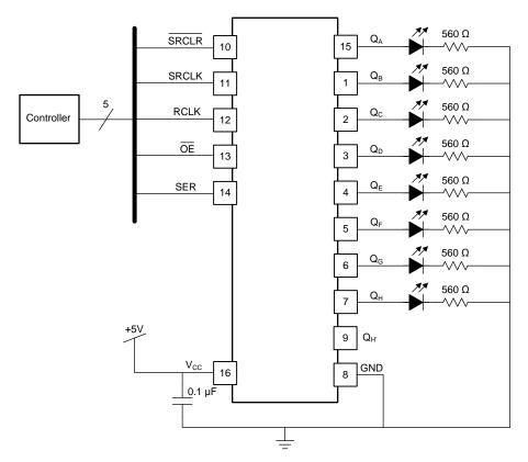
Figure 5. Typical Application Schematic
