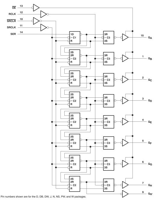
Figure 4. Logic Diagram (Positive Logic)
