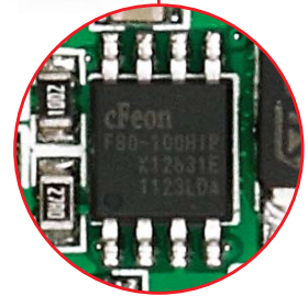
Figure 11-2: Flash memory module
