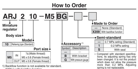
1) Backflow function is not available for standard. X209 is with backflow function.
