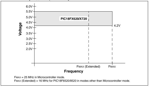
FIGURE 26-4: PIC18LF6620/6720/8620/8720 VOLTAGE-FREQUENCY GRAPH (INDUSTRIAL)
