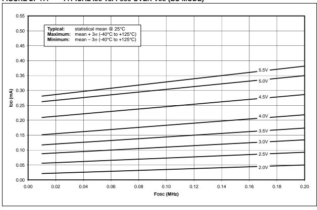
FIGURE 27-18: MAXIMUM IDD vs. Fosc OVER VDD (EC MODE)
