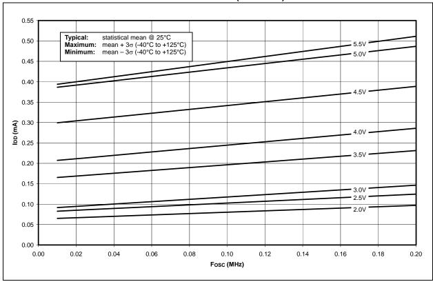
FIGURE 27-19: TYPICAL IDD vs. FOSC OVER VDD (EC MODE) (PIC18F8520 DEVICES ONLY)
