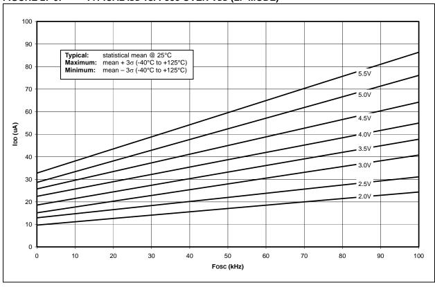
FIGURE 27-10: MAXIMUM IDD vs. Fosc OVER VDD (LP MODE) INDUSTRIAL
