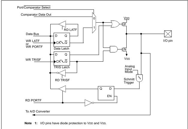
FIGURE 10-14: RF6:RF3 AND RF0 PINS BLOCK DIAGRAM
