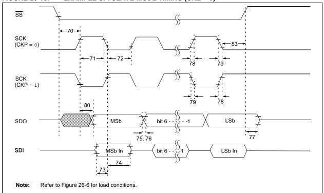
TABLE 26-17: EXAMPLE SPI MODE REQUIREMENTS (SLAVE MODE TIMING, CKE = 0)
