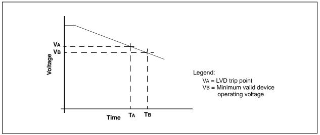
The block diagram for the LVD module is shown in Figure 22-2. A comparator uses an internally generated reference voltage as the set point. When the selected tap output of the device voltage crosses the set point (is lower than), the LVDIF bit is set.
