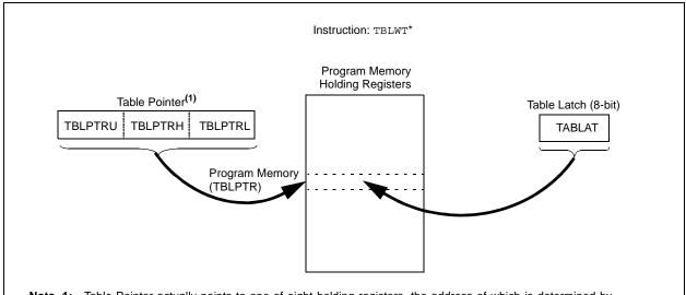
Note 1: Table Pointer actually points to one of eight holding registers, the address of which is determined by TBLPTRL<2:0>. The process for physically writing data to the Program Memory Array is discussed in Section 5.5 "Writing to Flash Program Memory".
