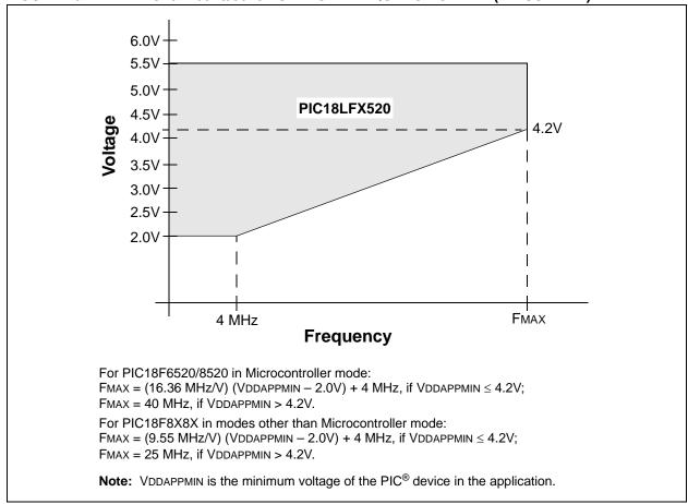
FIGURE 26-3: PIC18F6620/6720/8620/8720 VOLTAGE-FREQUENCY GRAPH (INDUSTRIAL, EXTENDED)
