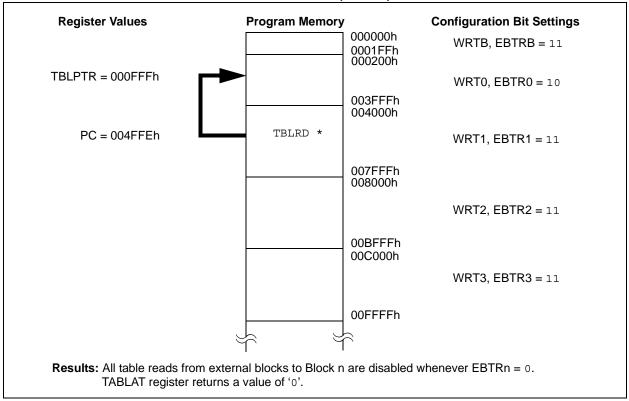
FIGURE 23-7: EXTERNAL BLOCK TABLE READ (EBTRn) ALLOWED
