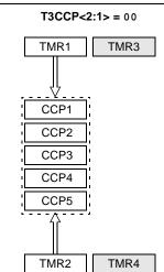
Timer1 is used for all Capture and Compare operations for all CCP modules. Timer2 is used for PWM operations for all CCP modules. Modules may share either timer resource as a common time base
