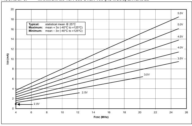
FIGURE 27-4: TYPICAL IDD vs. Fosc OVER VDD (HS/PLL MODE)
