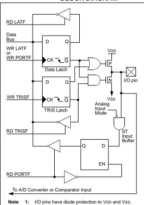
FIGURE 10-15: RF7 PIN BLOCK DIAGRAM
