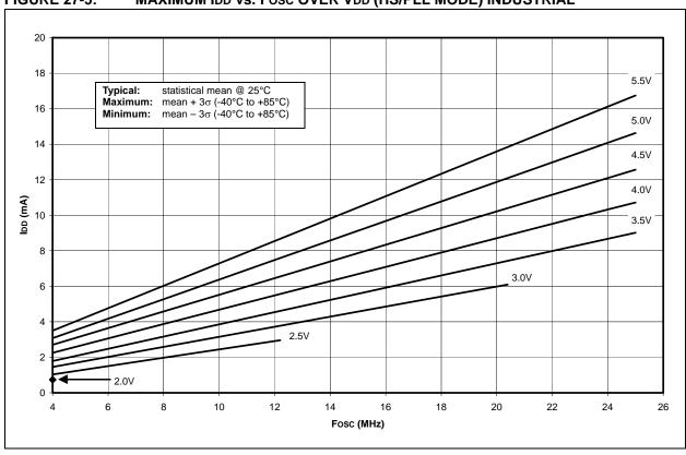
FIGURE 27-6: MAXIMUM IDD vs. FOSC OVER VDD (HS/PLL MODE) EXTENDED
