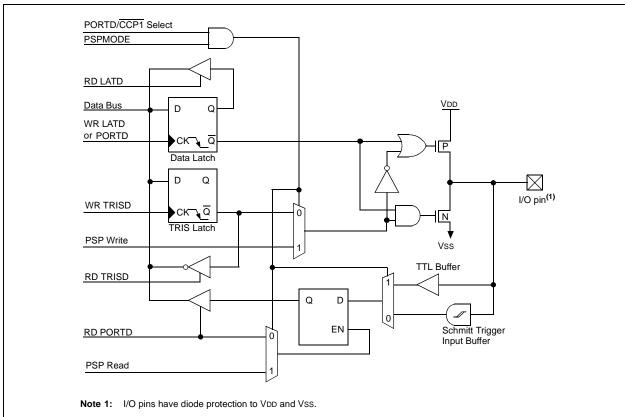
FIGURE 10-10: PORTD BLOCK DIAGRAM IN SYSTEM BUS MODE
