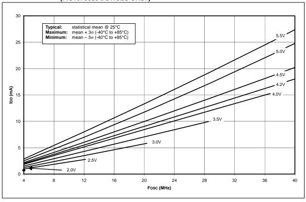
FIGURE 27-21: MAXIMUM IDD vs. Fosc OVER VDD (EC MODE) EXTENDED (PIC18F8520 DEVICES ONLY)
