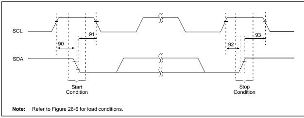
TABLE 26-19: I<sup>2</sup>C BUS START/STOP BITS REQUIREMENTS (SLAVE MODE)
