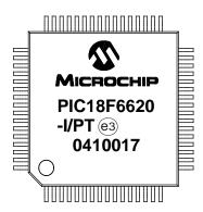
80-Lead TQFP (12x12x1 mm)
