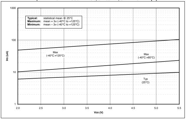
FIGURE 27-16: TYPICAL AND MAXIMUM AIWDT vs. VDD OVER TEMPERATURE (WDT ENABLED)
