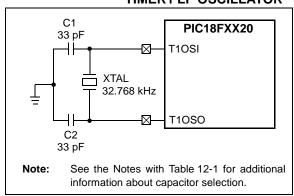
TABLE 12-1: CAPACITOR SELECTION FOR THE ALTERNATE OSCILLATOR
