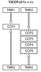
Timer1 and Timer2 are used for Capture and Compare or PWM operations for CCP1 only (depending on selected mode).
