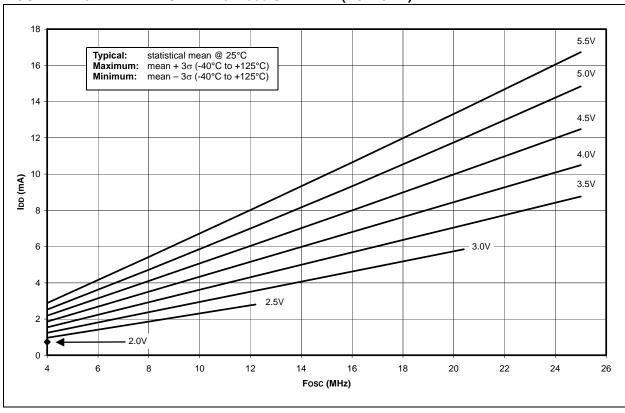
FIGURE 27-14: MAXIMUM IPD vs. VDD OVER TEMPERATURE
