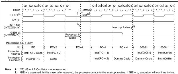
Tost = 1024 Tosc (drawing not to scale). This delay will not occur for RC and EC Oscillator modes.
