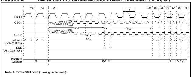
If the main oscillator is configured for HS-PLL mode, an oscillator start-up time (Tost), plus an additional PLL time-out (TPLL), will occur. The PLL time-out is typically 2 ms and allows the PLL to lock to the main oscillator
