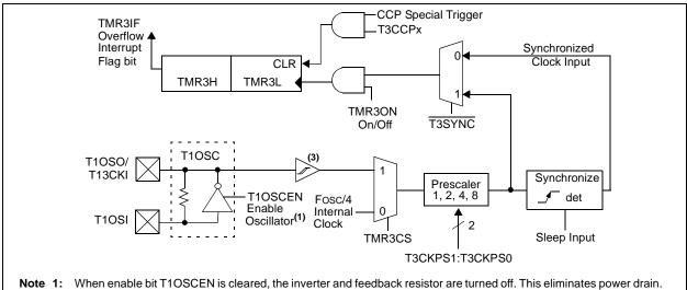
FIGURE 14-2: TIMER3 BLOCK DIAGRAM CONFIGURED IN 16-BIT READ/WRITE MODE
