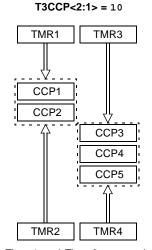
Timer1 and Timer2 are used for Capture and Compare or PWM operations for CCP1 and CCP2 only (depending on the mode selected for each module). Both modules may use a timer as a common time base if they are both in Capture/Compare or PWM modes.
