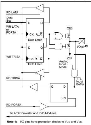
FIGURE 10-3: BLOCK DIAGRAM OF RA4/T0CKI PIN
