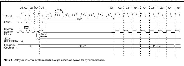
The sequence of events that takes place when switching from the Timer1 oscillator to the main oscillator will depend on the mode of the main oscillator. In addition to eight clock cycles of the main oscillator, additional delays may take place.
