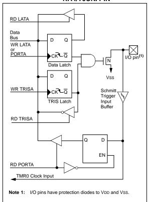
FIGURE 10-4: BLOCK DIAGRAM OF RA6 PIN (WHEN ENABLED AS I/O)
