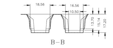
DIMENSIONS ARE IN MILLIMETERS [INCHES] WITH THE FOLLOWING TOLERANCES: [INCHES] ARE FOR REFERENCE ONLY. X.XX=  $\pm 0.25$  [ $\pm .010$ ]
