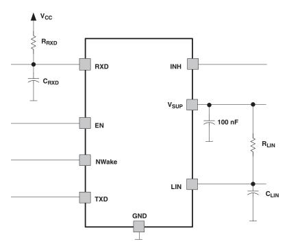
Figure 5. Test Circuit for AC Characteristics
