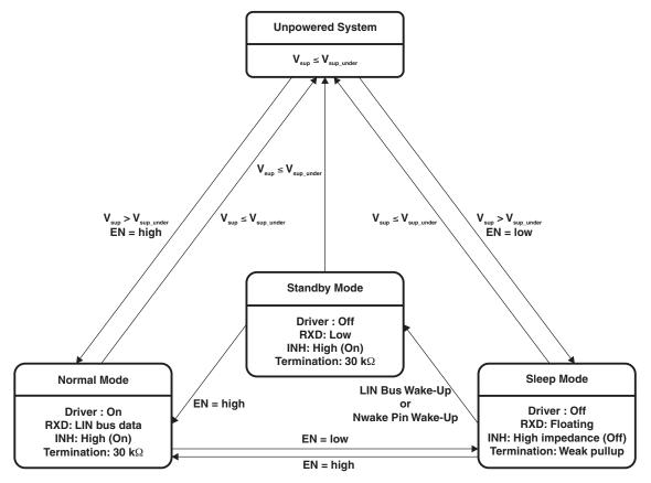
Figure 6. Operating States Diagram
