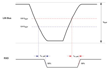
Figure 2. Propagation Delay
