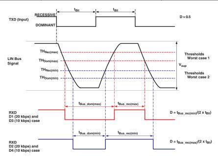
Figure 1. Definition of Bus Timing Parameters
