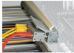
Testing with test plug modules.
