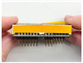
Since there's two modules and they don't sit completely flat on the PCB you may want to use a little tape to bind the modules together to minimize any gap in between.
