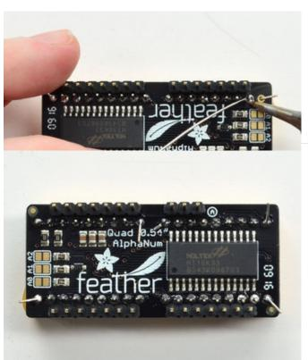
Check your solder joints visually and continue onto the next step
