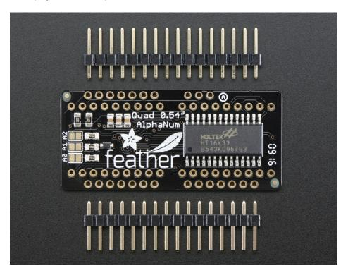
The LEDs themselves do not connect to the Feather. Instead, a matrix driver chip (HT16K33) does the multiplexing for you. The Feather simply sends i2c commands to the chip to tell it what LEDs to light up and it is handled for you. This takes a lot of the work and pin-requirements off the Feather. Since it uses only I2C for control, it works with any
