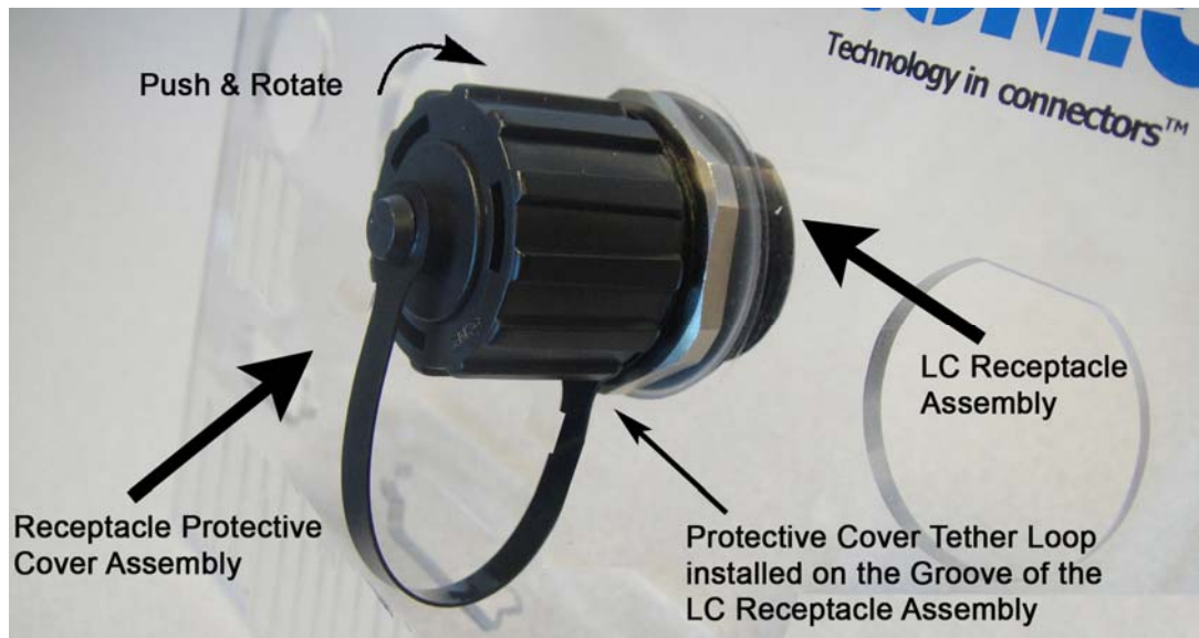
Figure 6-2: The Cover and Receptacle Adaptor Engagement
