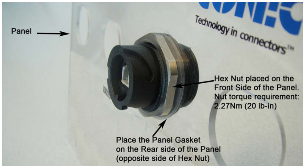
Figure 5-2: The Rear Panel mount
