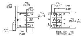
Actuator shown in pos. 1 - 'ON' position. SPST MODELS (D M14 & DM54) OMIT TERM INALS 2 & 2A.
