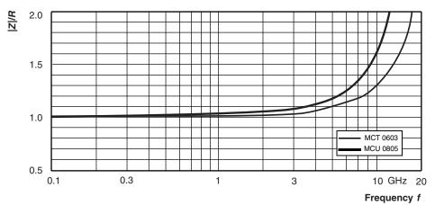
Relative impedance for 49.9  $\Omega$  chip resistor
