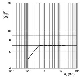
Maximum allowed peak pulse voltage in accordance with IEC 60065, 14.1.a; 50 discharges from a 1 nF capacitor charged to  $\hat{U}_{\text{max}}$ ; 12 discharges/min (drift  $\Delta R/R \leq 2$  %)
