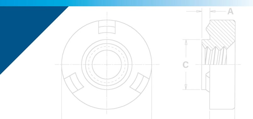
PEM<sup>®</sup> brand WN<sup>™</sup>/WNS<sup>™</sup> weld nuts are designed to be welded onto another metal surface into properly sized holes. The PEM<sup>®</sup> weld nut design helps overcome many problems associated with other welded nuts:
