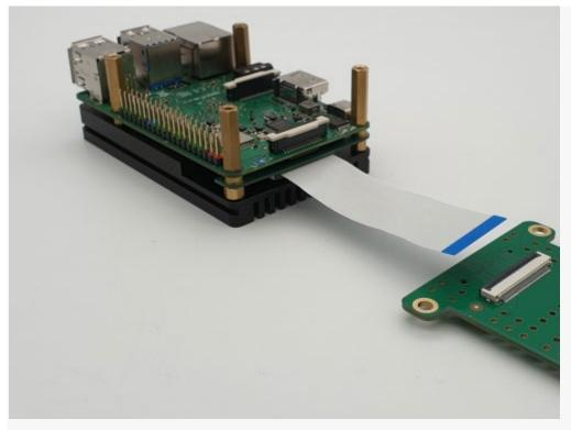
Open the FPC connector like before in lifting the black plastic part in the center.
