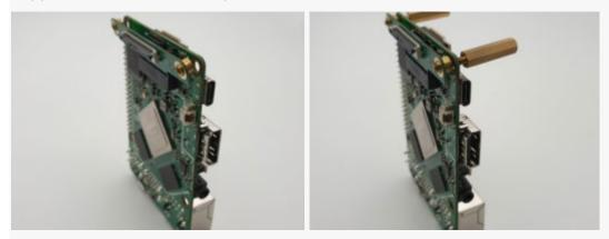
Now open the FPC connector in lifting the black part in the center up.
