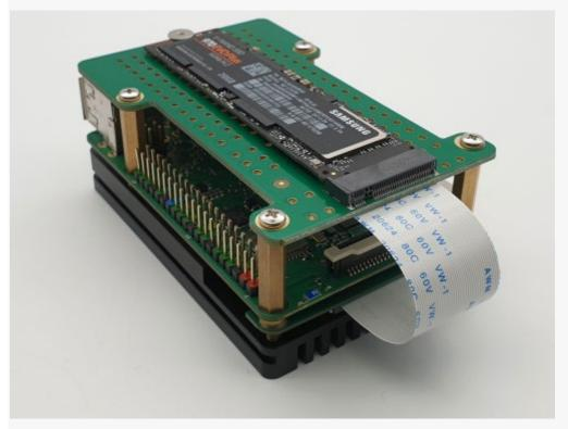
□NOTE – by default the FPC ribbon cable contacts should always face the PCB.
