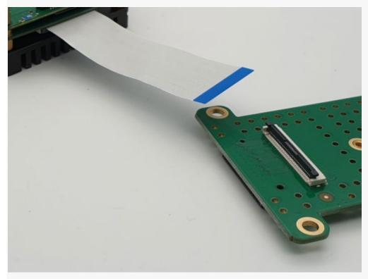
Insert the FPC ribbon cable and lock the connector in closing the black center part.
