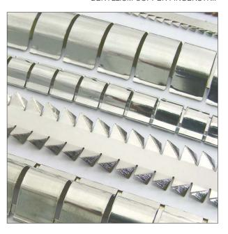
For maximum contact and shielding performance 25% compression is recommended. The standard finish is tin or bright copper, but special plating such as nickel or zinc with clear passivation can be specified to ensure galvanic compatibility. Fingerstrip can be ordered in Clean & Bright (C) or Tinned (T) as standard. Other finishes can be specified on request.
