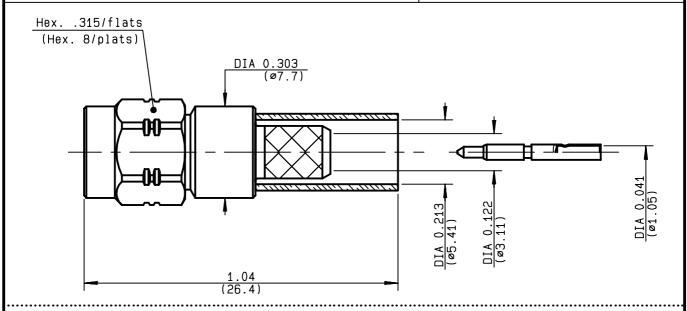
NOMINAL IMPEDANCE  $50 \, \Omega$ FREQUENCY RANGE  $0-12.4 \, \text{GHz}$
