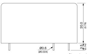
Dimensions in mm (inch) Tolerances:  $x.x \pm 0.5 (\pm 0.02)$
