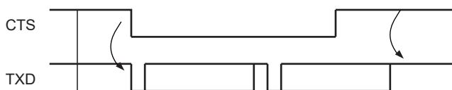
Figure 44-28. Transmitter Behavior when Operating with Hardware Handshaking
