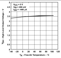
Only the 0°C to 70°C portion of the curve applies to the SN75176B device.
