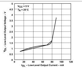
Figure 6-2. Driver Low-Level Output Voltage vs Low-Level Output Current
