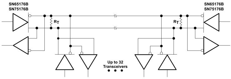
The line should be terminated at both ends in its characteristic impedance  $@_T = Z_O$ ). Stub lengths off the main line should be kept as short as possible.
