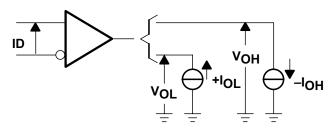
Figure 7-2. Receiver  $V_{OH}$  and  $V_{OL}$
