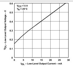
Figure 6-6. Receiver Low-Level Output Voltage vs Low-Level Output Current
