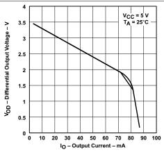
Figure 6-3. Driver Differential Output Voltage vs Output Current
