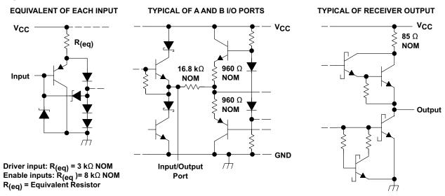
Figure 8-3. Schematics of Inputs and Outputs
