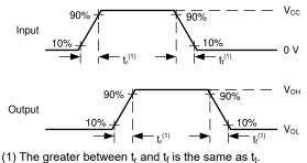
Figure 7-4. Voltage Waveforms, Input and Output Transition Times
