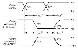
Figure 7-3. Voltage Waveforms Propagation Delays
