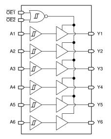
Figure 8-1. Logic Diagram (Positive Logic) for SN74HCS365-Q1
