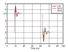
Figure 9-2. Simulated signal integrity at the reciever with different damping resistor (R<sub>d</sub>) values
