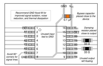
Figure 11-1. Example layout for the SN74HCS365-Q1 in the PW package.
