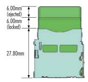
Short shell length and optimal card extraction length combine to offer space savings and easy card extraction.
