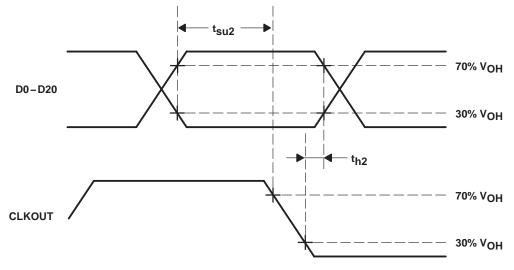
Figure 6. Setup and Hold Time
