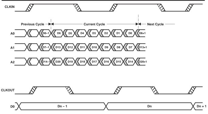
Figure 1. SN75LVDS86 Load and Shift Timing Sequences
