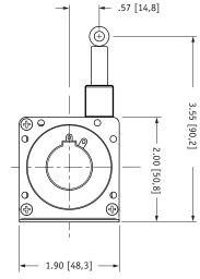
DIMENSIONS ARE IN INCHES [MM] tolerances are 0.04 IN. [1,0 MM] unless otherwise noted.
