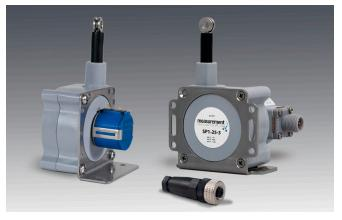
This compact stringpot with "voltage divider" output, provides ease-of-use and flexibility for measurement ranges up to 50 inches. Made of rugged polycarbonate, the SP1 fits in small spaces, doesn't need perfect alignment and ships with a stainless steel mounting bracket to let the user easily orient this sensor in just about any direction imaginable.
