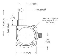
DIMENSIONS ARE IN INCHES [MM] tolerances are 0.04 IN. [1,0 MM] unless otherwise noted.
