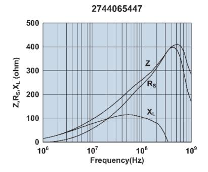
Impedance, reactance, and resistance vs. frequency.
