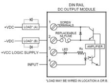
"LOAD MAY BE WIRED IN LOCATION A OR B. DC INDUCTIVE LOADS MUST BE DIODE SUPRESSED TO PREVENT DAMAGE TO THE I/O MODULE.
