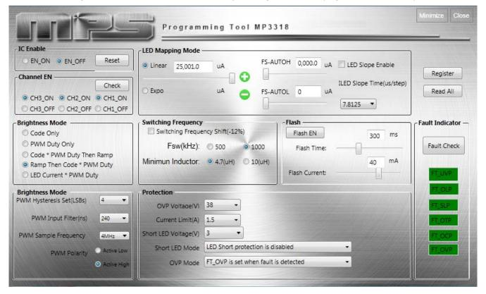
Figure 1: MP3318 MPS GUI Software
