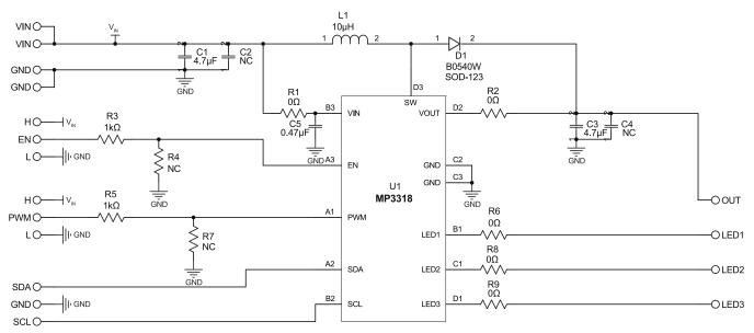
Figure 2: Typical Application Schematic with 3 strings (7 LEDs/string, 20mA/String)
