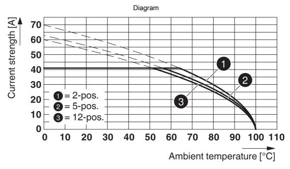
Type: SPC 5/...-STF-7,62 with DFK-PC 5/...-STF-7,62 Conductor cross section: 10 mm<sup>2</sup>
