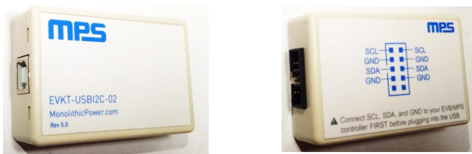
Figure 3: EVKT-USBI2C-02 Communication Interface
