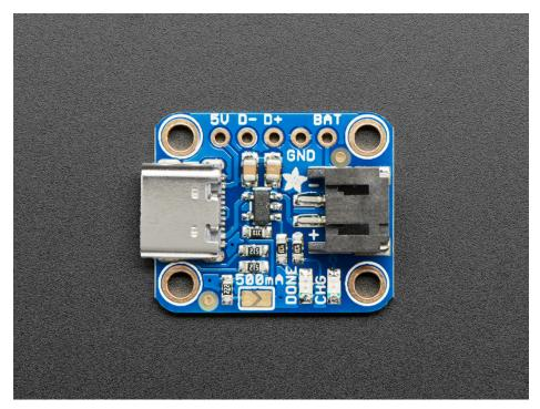
The USB-C Micro-Lipo charger is special. We've exposed the data lines so you can use it both as a USB-C breakout and a Micro-Lipo charger. Since there's a little more to it, we've included the pinouts here. Let's take a look!
