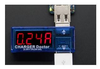
If you want to check the exact current draw during charge, try out a Charger Doctor between the USB port and charger. (https://adafru.it/dvm)
