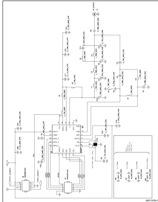
Figure 1: STEVAL-IKR002V1D circuit schematic
