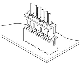
The ZH connector is very small with a mounting height of 5.6mm and a thickness of only 3.5mm. Contact retention lances on the housing make insertion easier, while the dimple at the center of the contact ensures reliable contact with the post.
